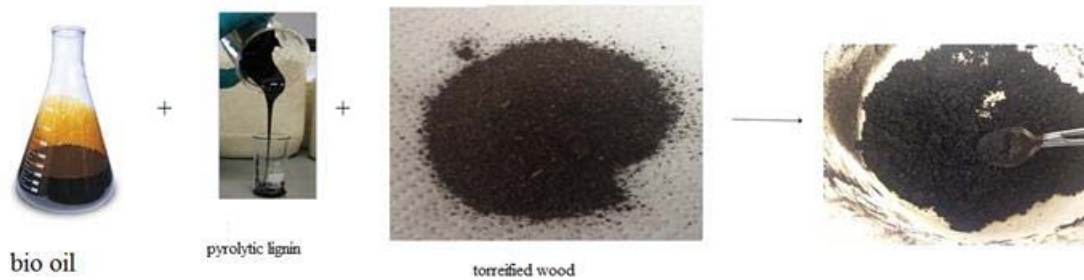
Figure 3.13 Mixing of bio oil, pyrolytic lignin and torrefied wood
